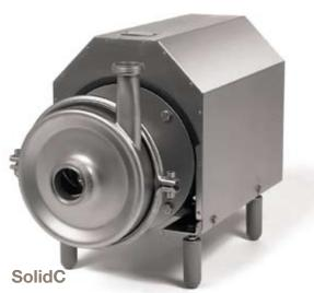
The SolidC pump series is a reliable and cost-effective solution for simple transport duties up to 85 m<sup>3</sup>/h. It utilizes the same mechanical shaft seal found in our LKH series, which is front-loaded and easily replaced without removing the backplate. SolidC pumps are available in four sizes and comply with 3A, CE and EHEDG requirements.
