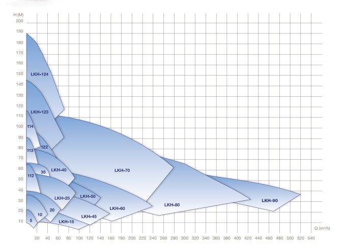
LKH performance LKH pumps are available for capacities up to 440 m<sup>3</sup>/h and pressures up to 190 m (19 bar/275 psi).
